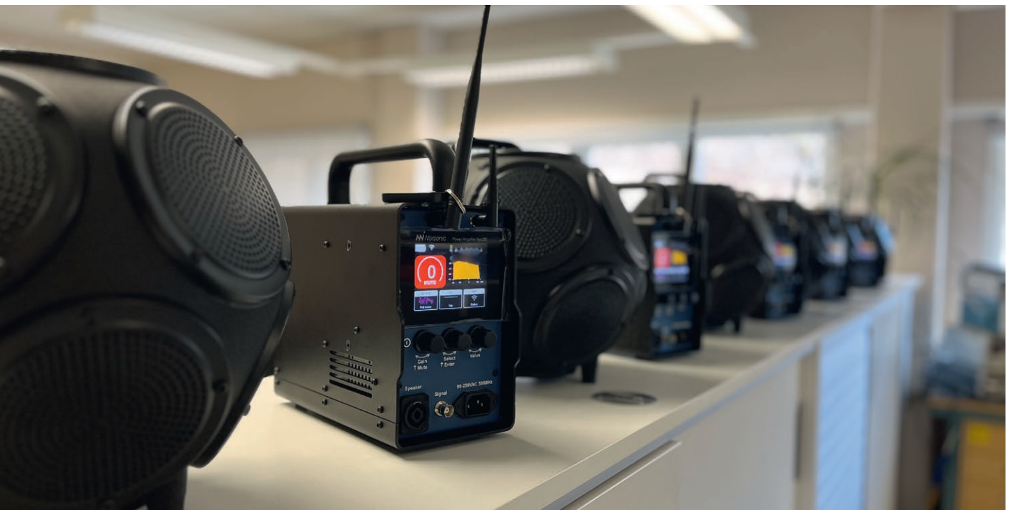
Nor283 dodecahedron loudspeakers and Nor282 power amplifiers ready for shipment.
